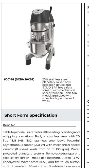
allows the mixer to switch on only when the bowl and the safety screen are properly installed and positioned together. Adjustable feet for stability. Supplied with 3 tools: spiral hook, paddle and whisk.
